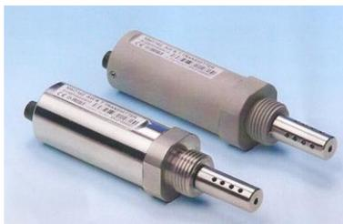
The MMT 162 probe leads are terminated in the Monitor enclosure, where the LCD display gives the local reading. SCADA connections are made using two analogue channel outputs for current and voltage giving readings for temperature and water in oil in ppm. The probes are fitted into stainless steel tee fittings which introduce the sensing head directly into the oil flow. The client must request the format in which the SCADA signals are to be presented.
