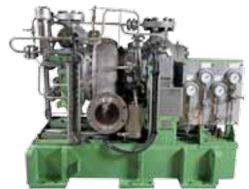
Turbine driven auxiliary feedwater pump
