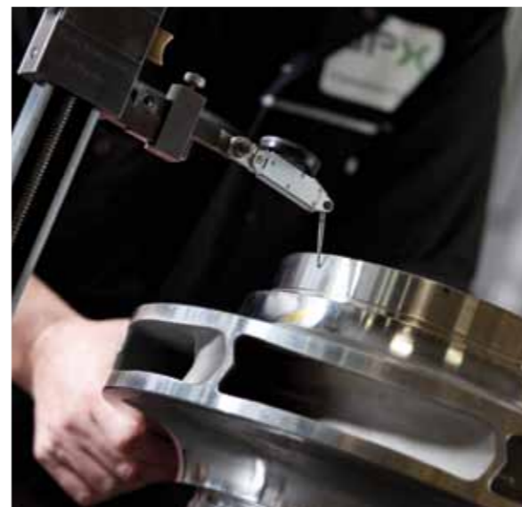
TOP - FINAL INSPECTION OF BRONZE IMPELLER
